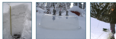
Fig. 5: From left to right: Snow profile with distinct layering; chamber for CO 2 flux measurements on the snow surface; Aluminum snow probe for CO 2 concentration profile measurements.
